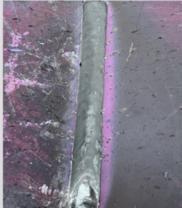
Test weld seam(base+fill+cover, solid core welding wire)
