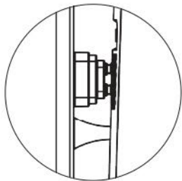
Full contact of metal sheet
